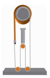
The EFAFLEX wind load system provides permanent door leaf tension. Perfect where wind or negative pressure causes a draft!
