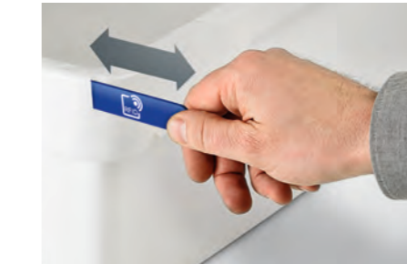
Traceability via retrofitable RFID (UHF) transponder
